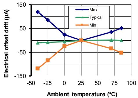
Figure 5: Electrical offset thermal drift
