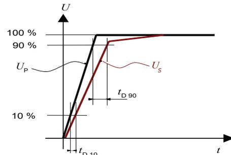
Figure 15: Delay time  $t_{D10}$  @ 10 % and delay time  $t_{D90}$  @ 90 %.
