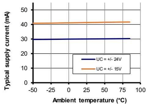
Figure 3: Supply current function of temperature
