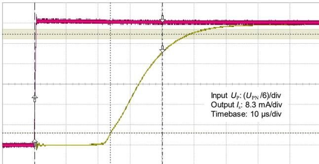
Figure 10: Typical step response (0 to  $U_{PN}$ )
