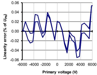
Figure 7: Typical linearity error at 25 °C
